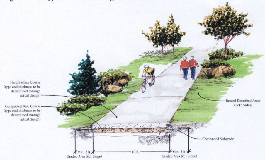
Figure 4.5.1. Typical Hard-Surfacing Cross-Section
